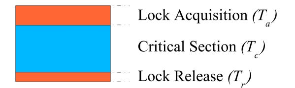
$$Efficiency = \frac{T_c}{T_c + T_a + T_r}$$
